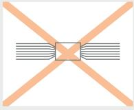
Crushing the individual cables is to avoid when assembling them into bunches.
