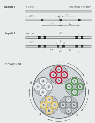
The tracer bunch is identified by a red plastic spiral in every layer. The other bunches have a white spiral. The quads of a primary bunch are counted in the order of the basic colours.
